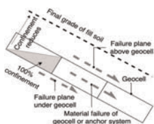
Figure 1a. Modes of failure.
