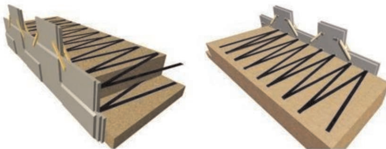
Figure 2. Typical of geoforce segmental retaining wall system.
