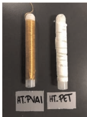
Figure 5. Comparison between PVAI and PET yarn exposed to a saturated lime solution at 80°C.
