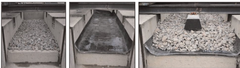
Figure 5. Vibrogyr testing simulating rail traffic on ballast by SNCF (French Railways).
