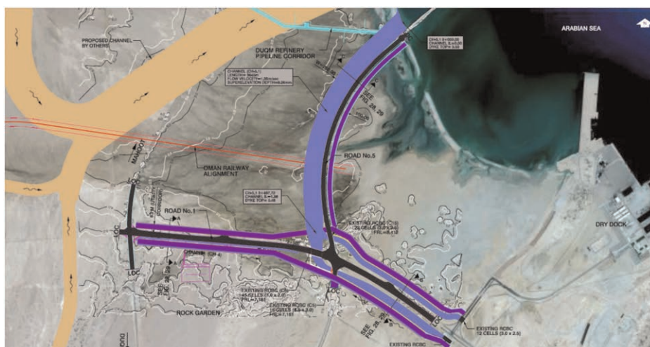
Figure 5. Plan view of road network and drainage channels in Duqm roads project.
