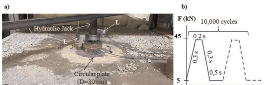
Figure 2. a) Plate load test setup, b) Cycles applied.
