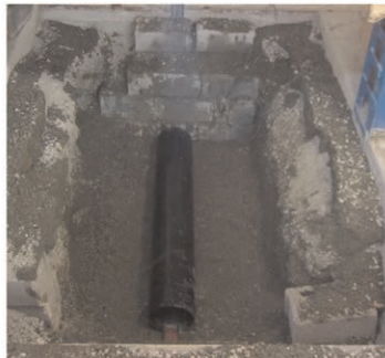
Figure 21. (a & b) Schematic installation of LVDTs inside the pipe, (c & d) Photograph view of pipe and steel U channel solid base, magnet base/rod and LVDTs inside the pipe (Moghaddas Tafreshi et al. 2020).
