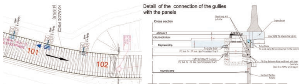
Figure 4. T6A-T6M ramp: (a) Plan view of geostrips layout; (b) detail of connection of gully with panels.
