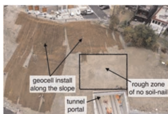
Figure 4. Layout of the slope with tunnel portal.
