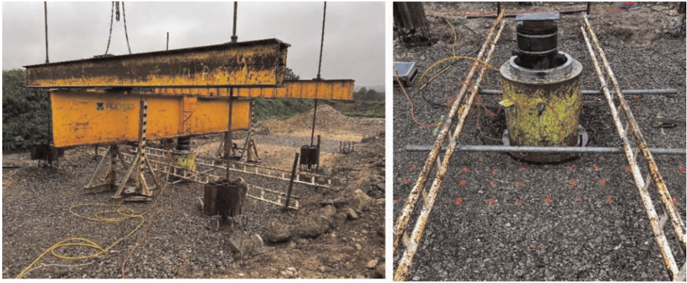
Figure 4. Left: Reaction frame; Right: Load cell.
