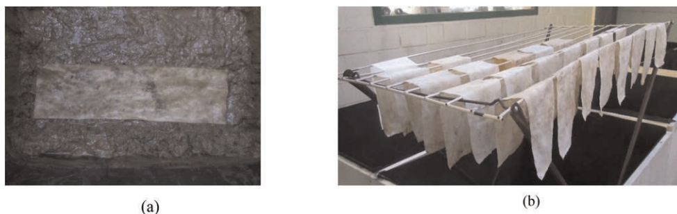
Figure 1. Photos for soil burial test (a) buried sample, and (b) dried samples.
