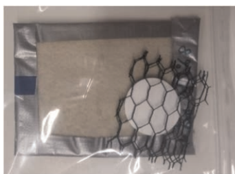
Figure 1. Filter paper setup for measuring total suction.
