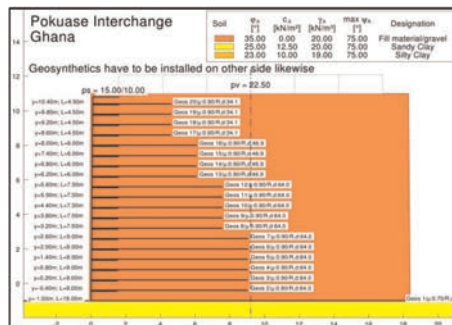
Figure 3. Layout and input parameters for stability analysis in GGU Stability software.
