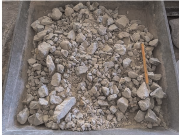
Figure 5. Overliner material used in large scale puncture test.
