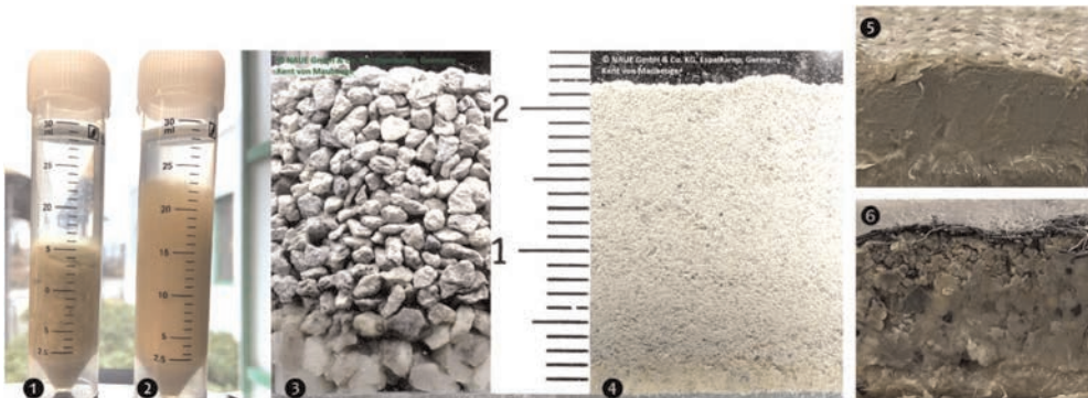
Figure 3. Free swell of solely 1g of granular (1) and powder (2) bentonite – granular bentonite (3), granular bentonite GCL (6) powder bentonite (4) and powder bentonite GCL (5) hydrated from the bottom for 24h (powder bentonite closes pores immediately, while granular bentonite still shows several open pores).
