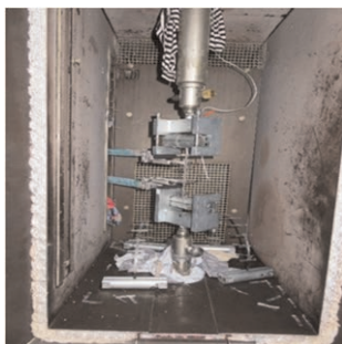
Figure 5. Single rib tensile testing in a temperature-controlled chamber.
