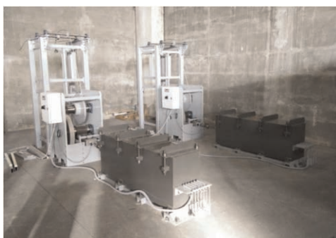
Figure 1. Large-scale prototype apparatus for long-term pullout tests.
