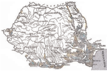
Figure 1. Collapsible soil spreading in Romania (NP 125:2010).
