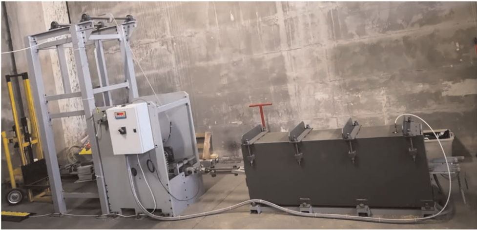
Figure 11. Large-scale prototype apparatus for long-term pullout tests.
