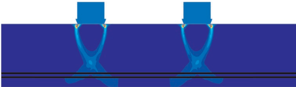
Figure 5. Failure within a thicker working platform with insufficient shear strength ( h_{\text{platform}}=2\text{ m} , \varphi_p=27^\circ ).
