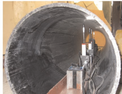
Figure 21. (a & b) Schematic installation of LVDTs inside the pipe, (c & d) Photograph view of pipe and steel U channel solid base, magnet base/rod and LVDTs inside the pipe (Moghaddas Tafreshi et al. 2020).
