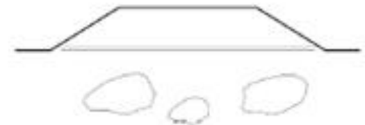
Reinforcement over areas prone to subsidence
