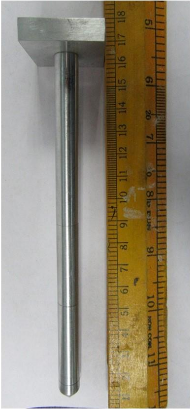
END BEARING PILE
