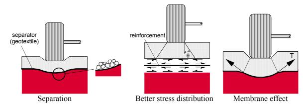
Influence of geosynthetic reinforcement on unpaved road behaviour
