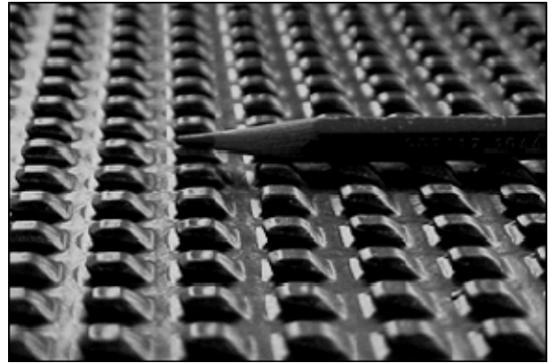
Figure 31: Cuspated GCD geometry after loading to 300 kPa
