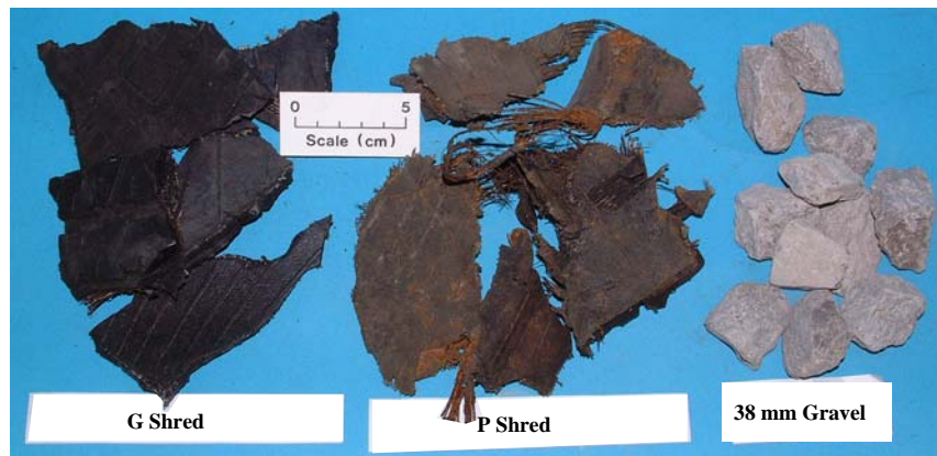
Figure 6. Tire shred and 38mm gravel considered by McIsaac and Rowe (2005) and Rowe and McIsaac (2005)
