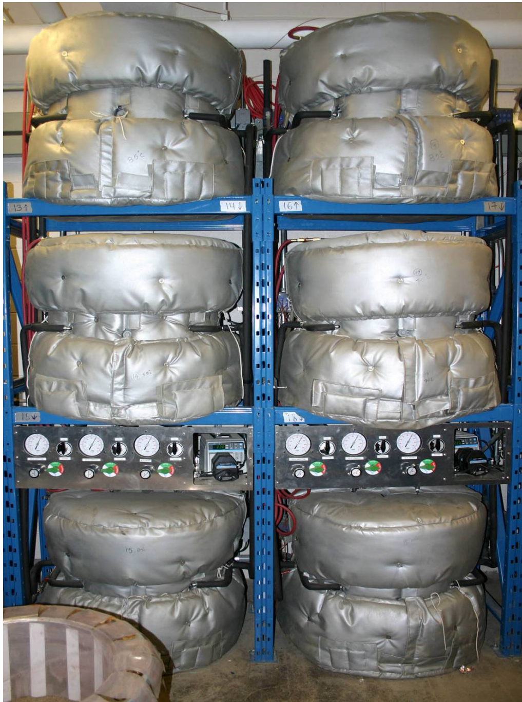
Figure 8. Photograph of six GLLSs tests in progress and an additional one (lower left) being assembled.
