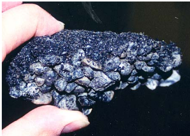
Figure 5. Concreted zones of cemented sand and cemented pea gravel. Reproduced from Mclsaac, R. and Rowe, R.K. (2006) Effect of filter/separators on the clogging of leachate collection Systems, Canadian Geotechnical Journal , 43 (7): 674-693 with permission of the Canadian Geotechnical Journal.
