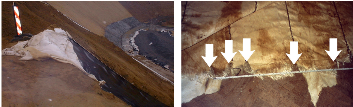
Fig. 11. The failure of the reinforcement geotextile at the top of the slope.
