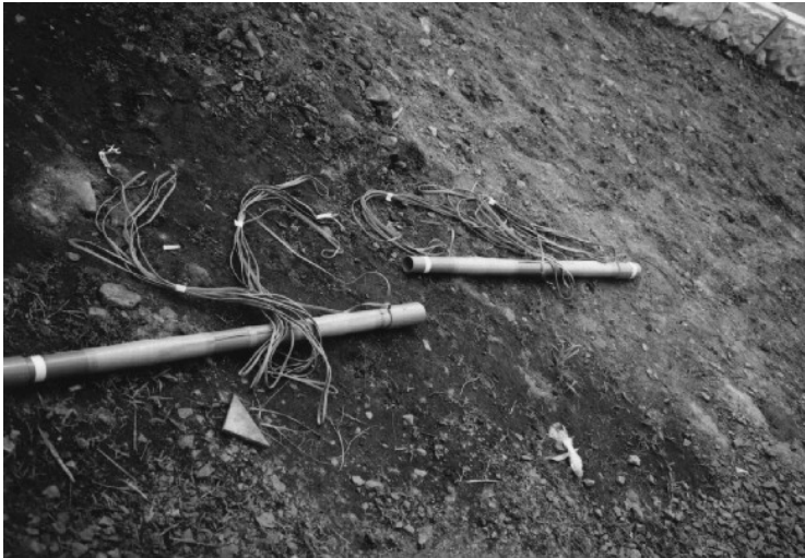
Photo-6 Inclinometer (pipe gage)
