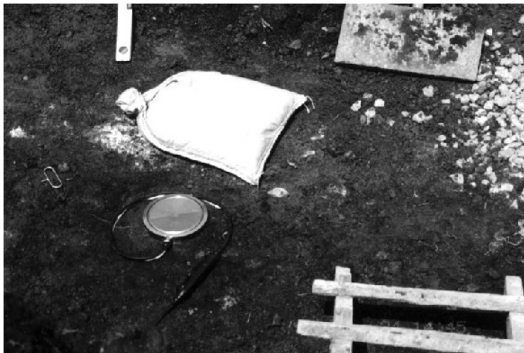
Photo-2 Earth pressure gauge (vertical direction)
