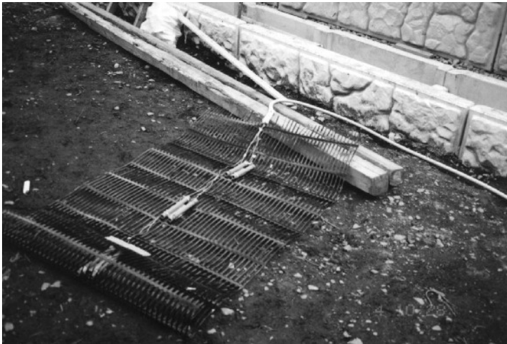
Photo-4 Strain gauge (7 layers: 34 in amount)
