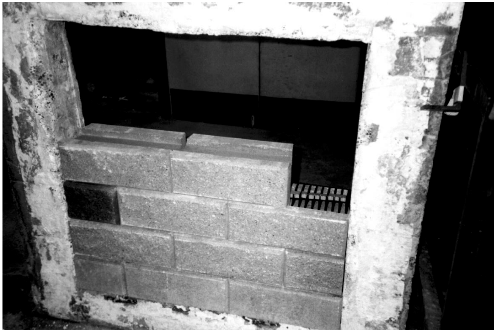
Figure 13. 1m x 1m. unit ready to be offered up to the furnace
