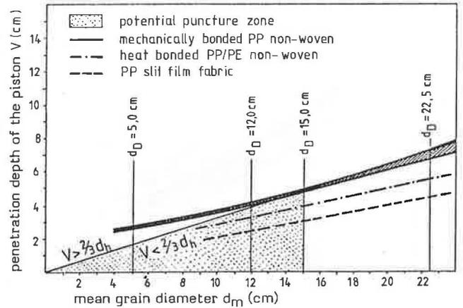
Fig. 6: Design chart II for puncture strength
