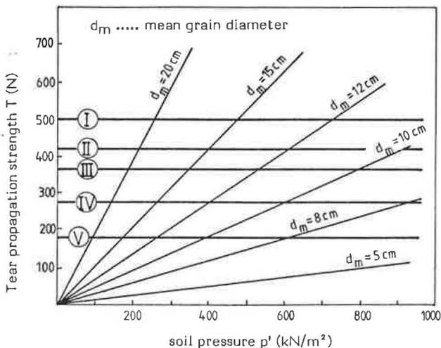
Fig. 10 Design Chart V for tear propagation strength (2)
