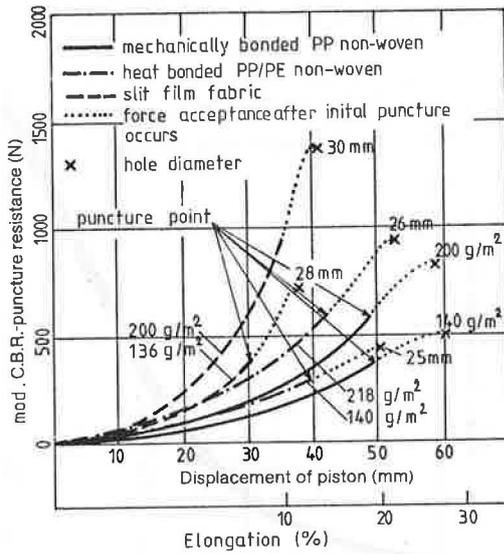
b) comparison of mechanically bonded and heatbonded non-woven and slit-film geotextiles
