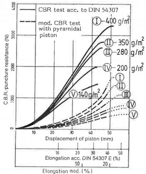
Fig. 4: Force -elongation diagram for
