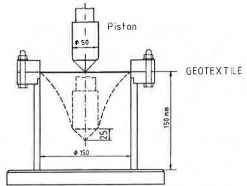
Fig. 3: Modified CBR test
