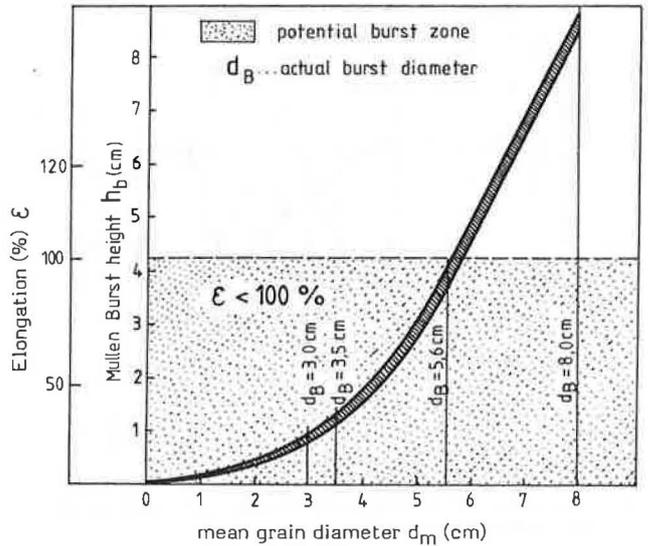
Fig. 8 Rating diagram IV for burst elongation
