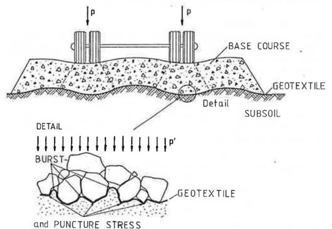
Fig. 1 Geotextile stresses decisive for the separation function
