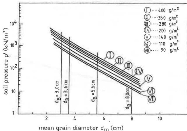
Fig. 7 Design Chart III for bursting strength
