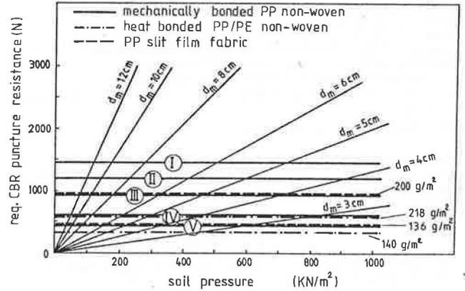
Fig. 5: Design Chart I for puncture strength
