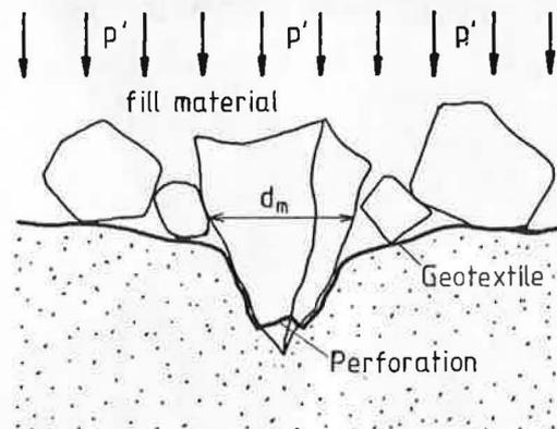
Fig. 9 Tear propagation stress of a geotextile
