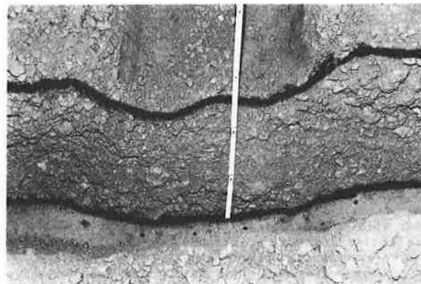
Fig. 9: Trackings in the surface (dual wheels, dolomite surface), wheelers in the subsoil ("Loess" subsoil, needle punched nonwoven)
