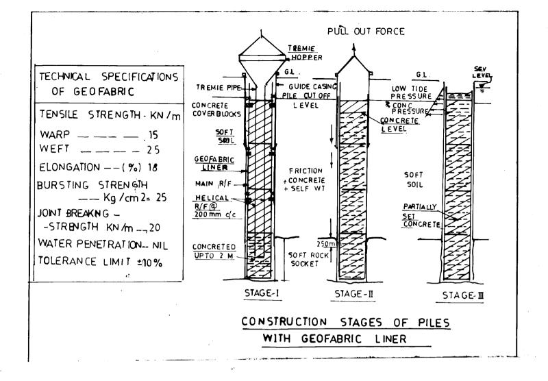
bursting of geofabric. There was ample evidence of bursting type of failure, provided by exposed piles.
