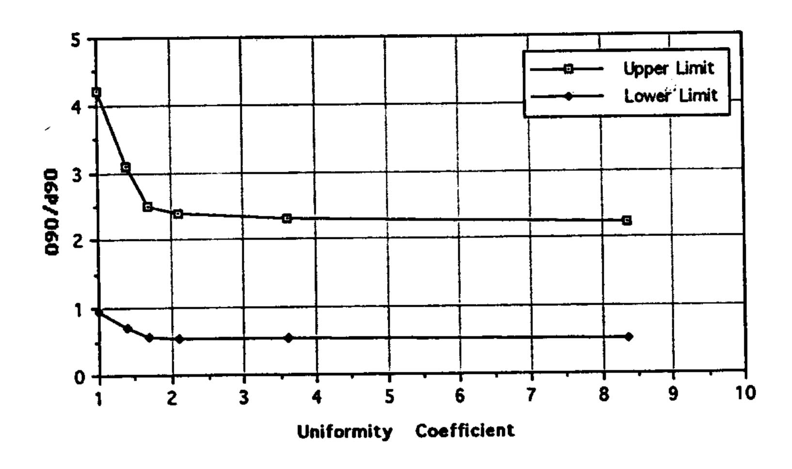
Fig. 2 Filter design criteria for non-compressible geotextiles with unidirectional flow
