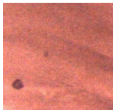
Fig. 4 Morphological image of the biggest carbon black particle and carbon black agglomerate in specimen 3 # made by microtome
