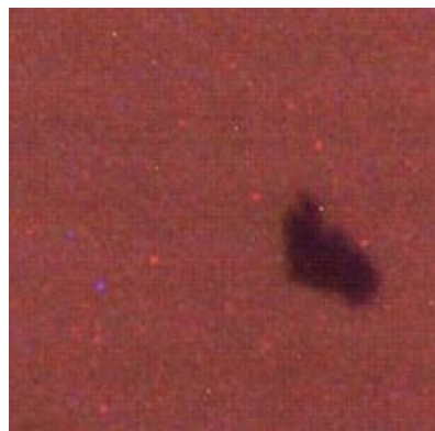
Fig. 2 Morphological image of the biggest carbon black particle and carbon black agglomerate in specimen 4 # made by compressing
