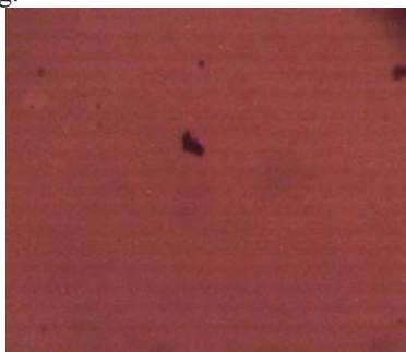
Fig. 1 Morphological image of carbon black particles and carbon black agglomerates in specimen 4 # made by compressing
