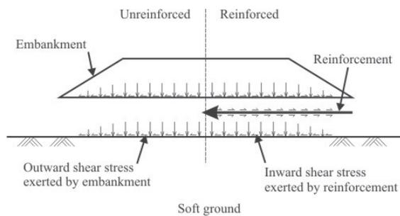
Fig. 1 A summary of reinforcement mechanics of an embankment on soft ground (adapted from Jewell, 1996)
