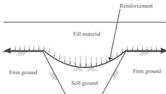
Fig. 2 A summary of reinforcement mechanics of a differentially deforming foundation subject to uniform vertical loading
