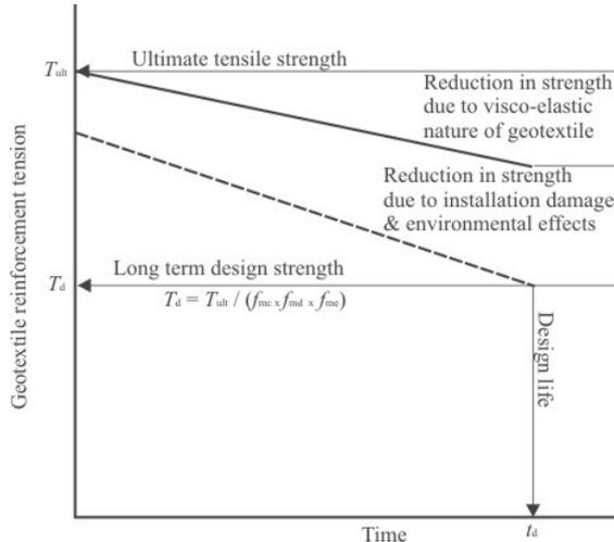
Fig. 4 Methodology used to derive the long term design strength of geotextile reinforcement
