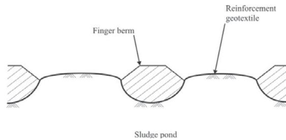
Fig. 3 Tensioned membrane effect due to differential deformation resulting from the load imposed by the finger berm above
