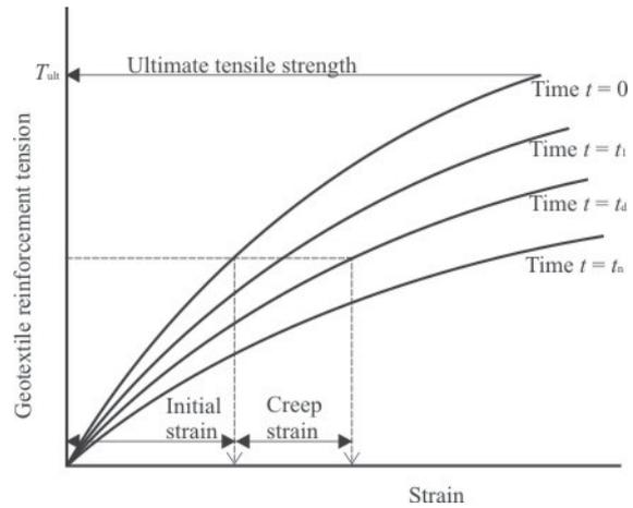
Fig. 5 Typical isochronous creep curves for geotextile reinforcements
