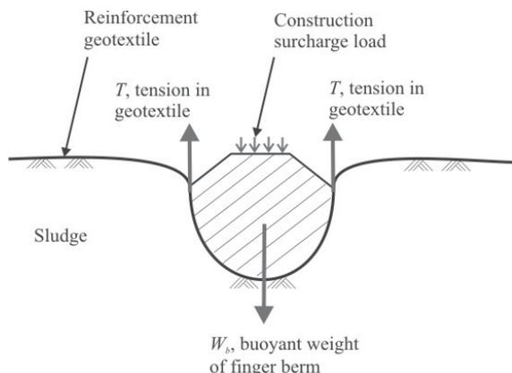
Fig. 10 The force diagram for the determination of the tension in the reinforcement
