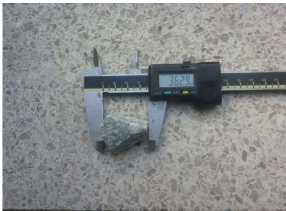
Fig. 3 Maximum particle size of filler
