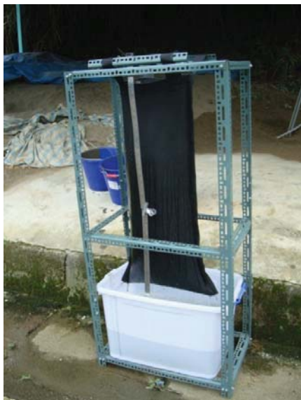
Fig. 4 Illustration of the hanging bag test
