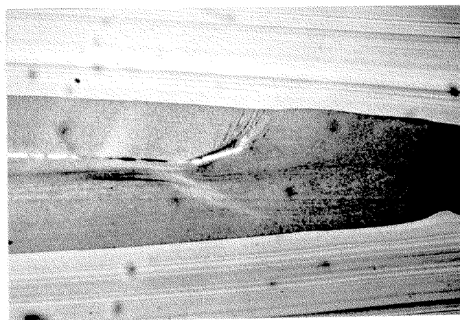
Figure 4 Photomicrograph of the COEX Seam Tested for Stress Crack Resistance (Magnification - 40X)
