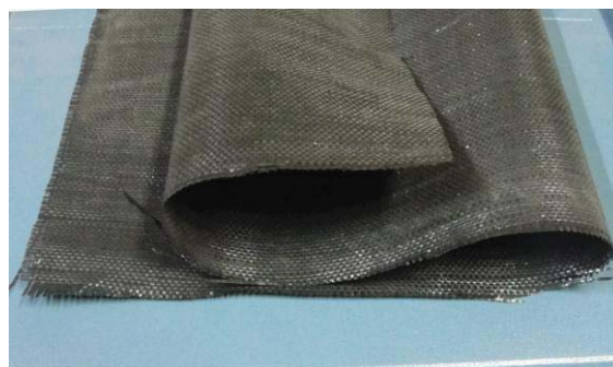
Fig. 1 A view of the woven geotextile (WGT)
