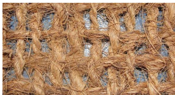
Fig. 2 A view of the coir geotextile (CGT)
