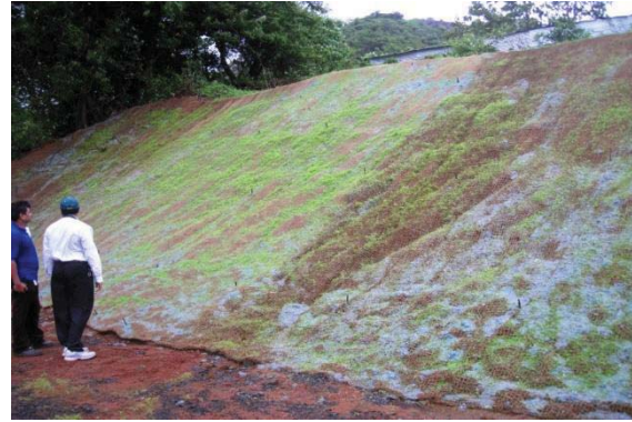
Fig. 12 A comparative performance evaluation of hydroseeding over woven and nonwoven CCM geotextiles
