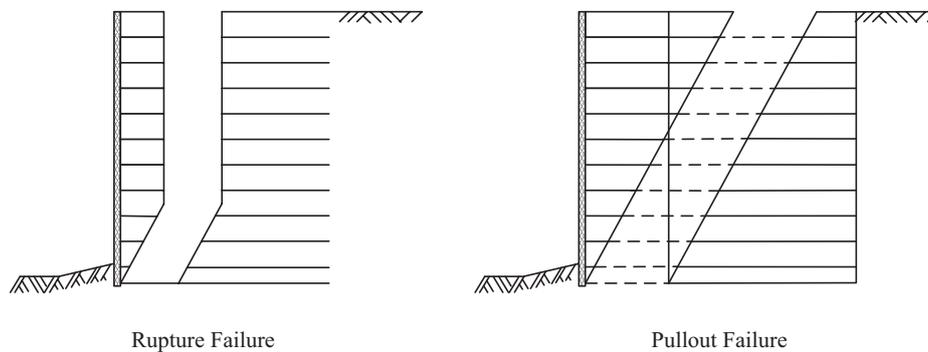
Fig. 5 Internal stability of reinforced earth wall
