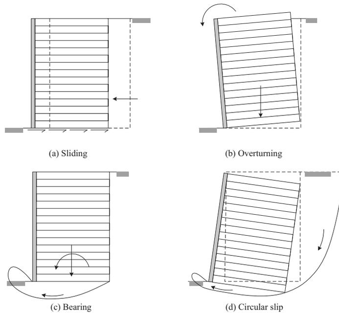
Fig. 4 External stability of reinforced earth wall
