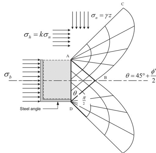
Fig. 7 Possible failure mechanism of a single isolated transverse member (Horpibulsuk and Niramitkornburee, 2010)
