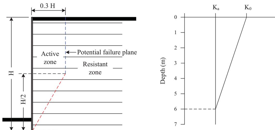
Fig. 6 Failure plane and approximate  $K$  for bearing reinforcement earth wall (Horpibulsuk et al., 2010 and 2011 and Suksiripattanapong et al., 2012)
