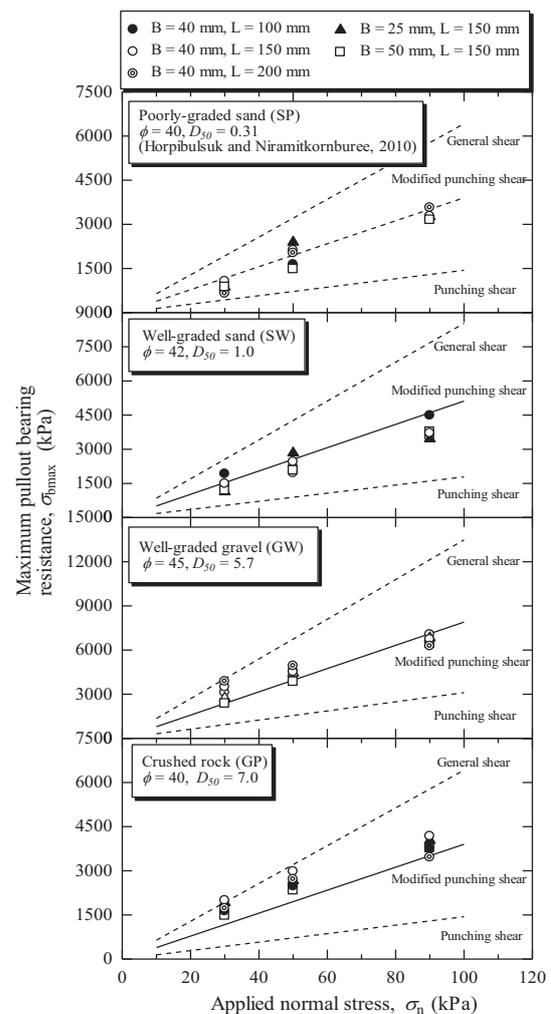
Fig. 8 Maximum pullout bearing resistance of a single isolated transverse member for all tested soils (Suksiripattanapong et al. 2012b).
