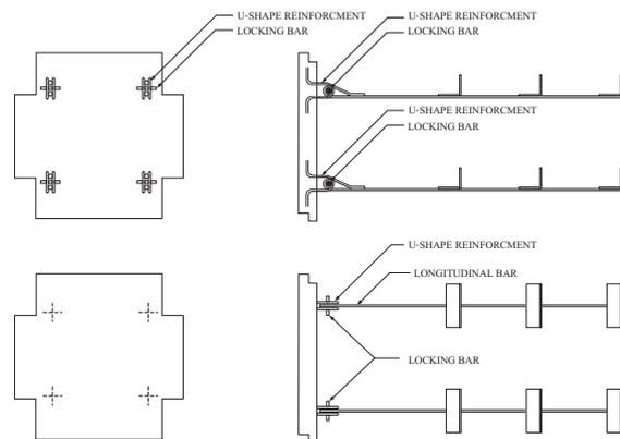
Fig. 2 Connection of the bearing reinforcement to wall facing
