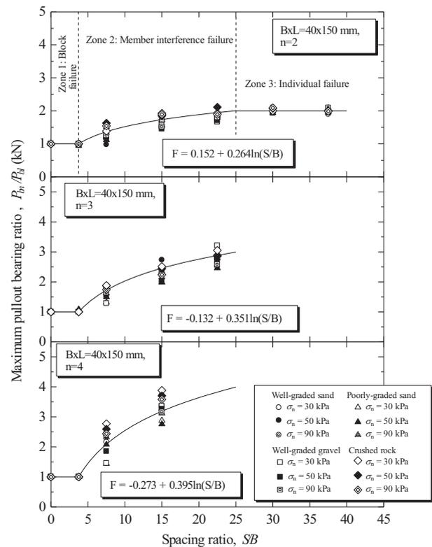
Fig. 9 Measured and predicted  $P_{bn}/P_{b1}$  and  $S/B$  relationship for 40x150 mm transverse members (Suksiripattanapong et al., 2012b).
