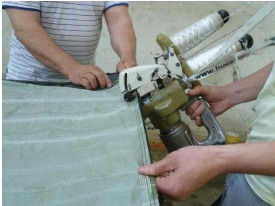
Fig. 5 Factory-made sewing of a panel.
