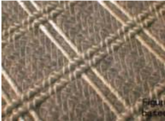
Fig. 4 Polyfelt PGM-G50/50 – nonwoven polypropylene geotextile reinforced with glass fibre.
