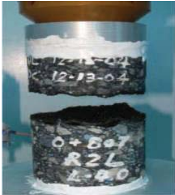
Fig. 7 Adhesion tests show paving fabrics improve bonding between layers.
