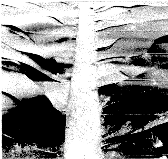
Fig. 23 Detail of central crack and shattering cracks branching from the central crack.
