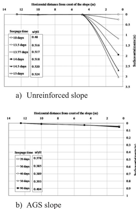
Fig. 7 Variation of measured surface settlements with the horizontal distance from crest of the slope (in prototype dimensions)
