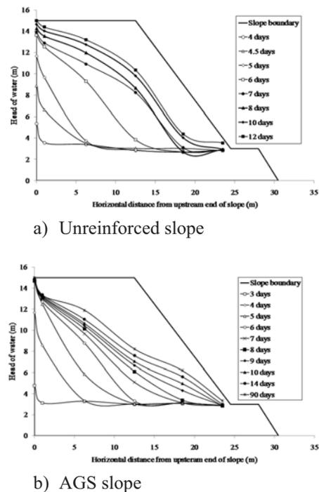
Fig. 8 Developed phreatic surfaces at various seepage times (in prototype dimensions)
