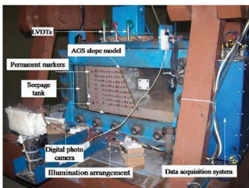
Fig. 3 View of developed AGS model before centrifuge test
