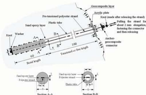
Fig. 1 Schematic diagram showing details of anchors of AGS (all dimensions are in mm)
