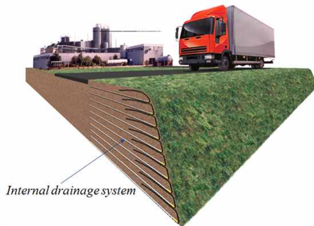
Fig. 3. Example of drainage at the back of the RSS and of internal drainage system
