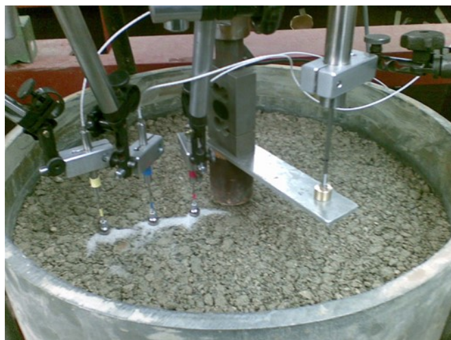
Figure 4. Loading on top of the surface of the base course
