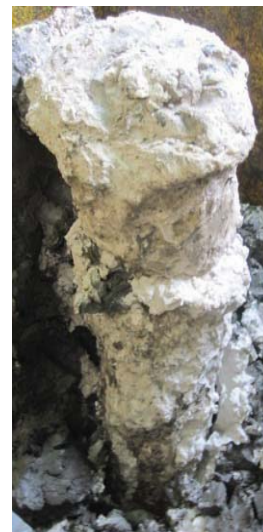
Fig. 12 Casted deformed shape of ordinary stone column.
