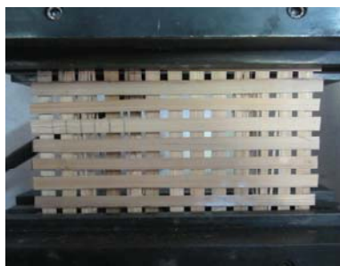
Fig. 3 Wide width bamboo grid specimen after tensile test
