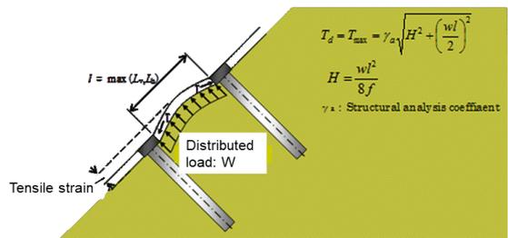
Figure 9. Cable theory to evaluate the ten-sile force Td in geocell.
