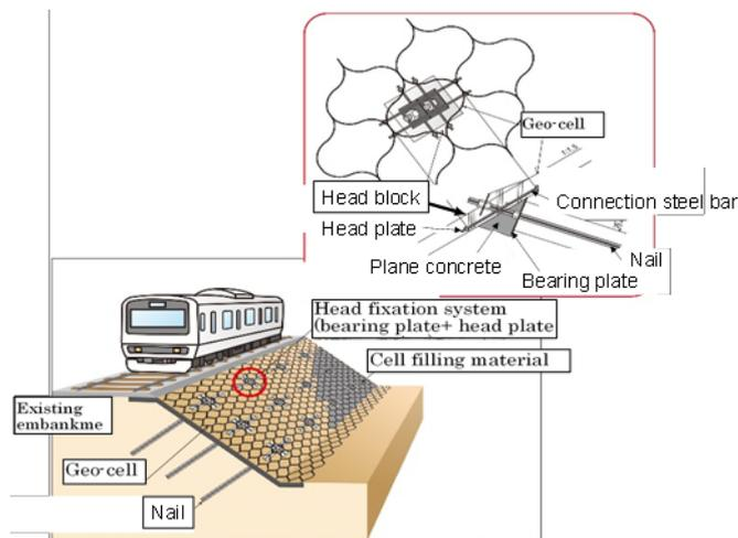
Figure 1. A new method to reinforce embankment slope
