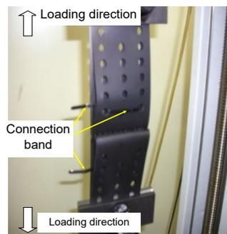
Figure 6. Tensile test on the geocell unit connection
