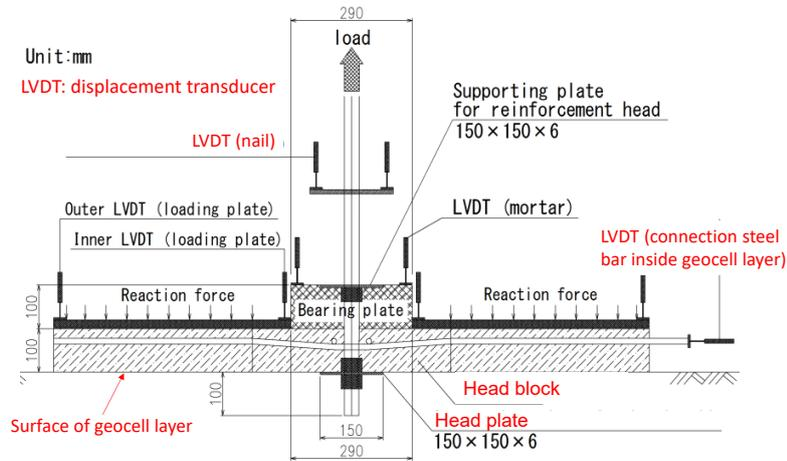
Figure 3. Loading test on geocell- nail connection
