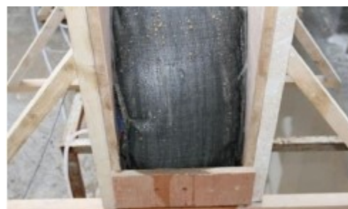
Figure 4. Geotube model filled by slurry
