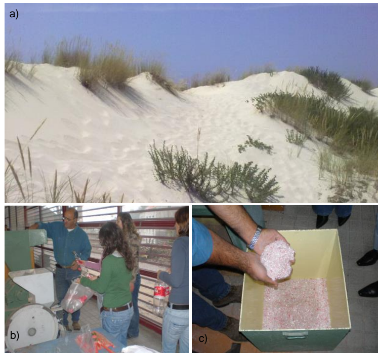
Figure 1. Materials in study: a) sand dune in nature; b) crushing the PET bottles; c) PET waste granulate.
