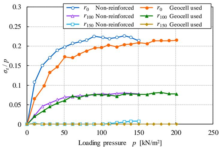
Figure 10. Relationship between  $\sigma_z / p$  and load pressure (state of layer thickness 150 mm)
