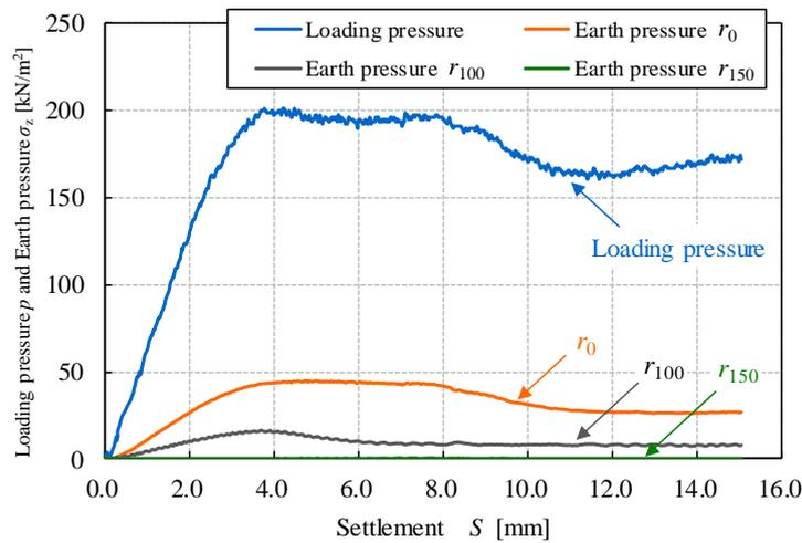
Figure 8. Load pressure Relationship between vertical stress in ground and settlement amount. (reinforcement)
