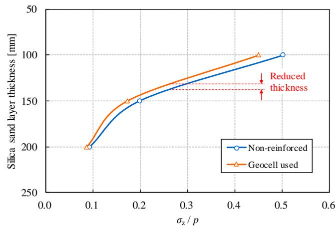
Figure 13. Relationship between the thickness of silica sand layer and  $\sigma_z / p$
