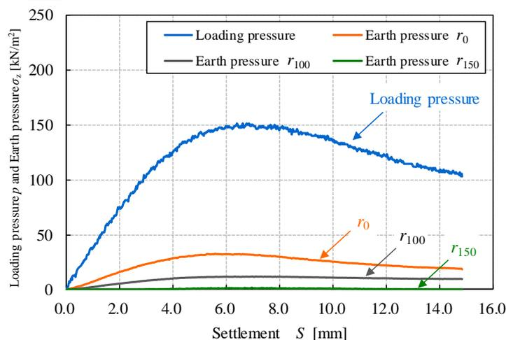
Figure 7. Load pressure Relationship between vertical stress in ground and settlement amount. (no reinforcement)
