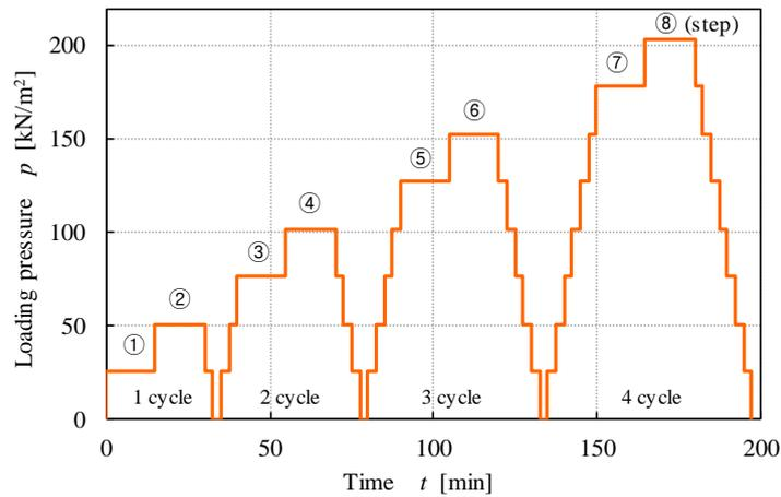
Figure 3 Loading condition of the step cyclic loading test
