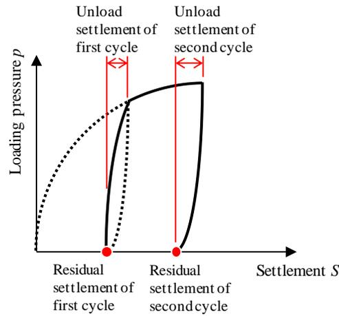
Figure 6. Definition of residual settlement amount and unloading amount.
