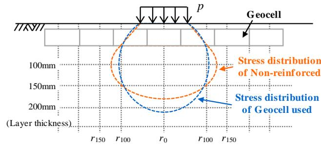
Figure 12. Schematic diagram of stress distribution by laying geocell
