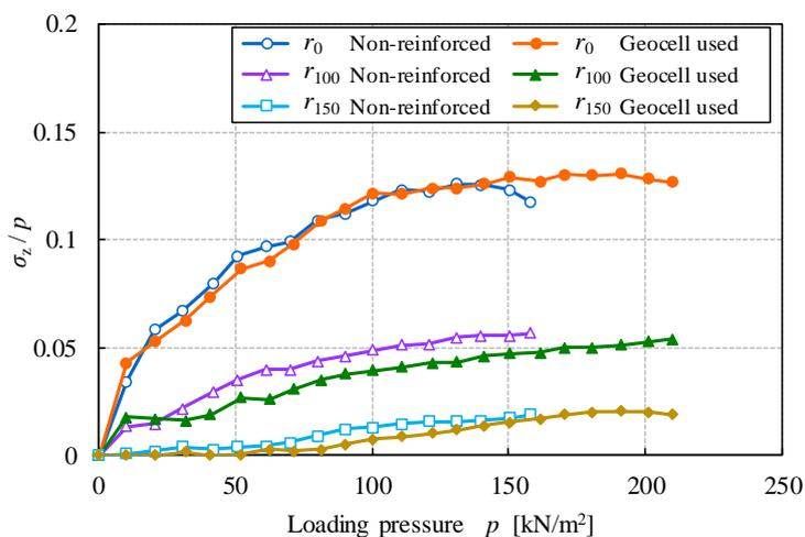
Figure 11. Relationship between  $\sigma_z / p$  and load pressure (state of layer thickness 200 mm)
