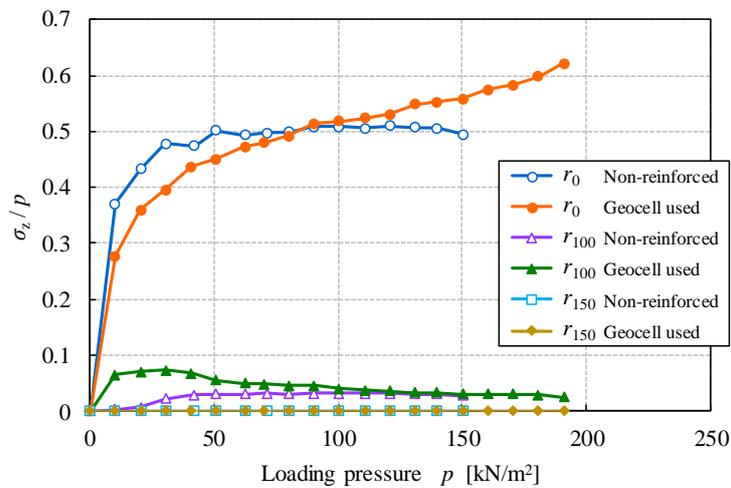
Figure 9. Relationship between  $\sigma_z / p$  and load pressure (state of layer thickness 100 mm)
