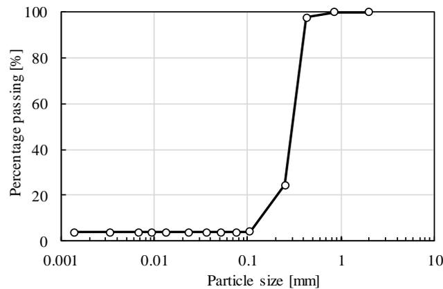
Figure 2. The grading curve of the silica sand
