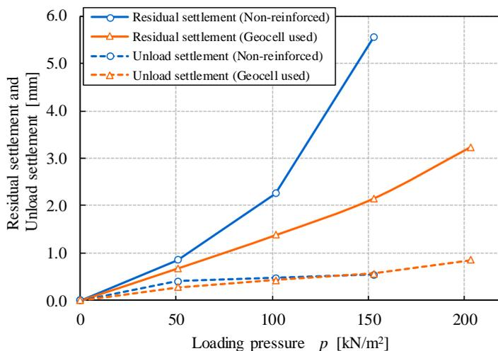
Figure 5. Relation between residual settlement and unloading settlement amount and loading pressure.
