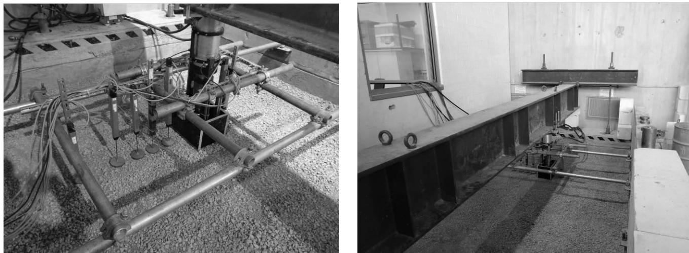
Figure 2: Setup of the model tests with actuator and potentiometric transducers (left) and testing field with reaction frame.
