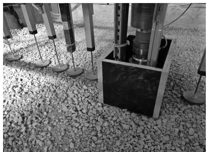
Figure 6: Comparison of the settlement of the load plate and on the surface on the reinforced and unreinforced support layer along the measuring cross section for unreinforced and reinforced supporting layers (left), arrangement of the potentiometric transducers (right).
