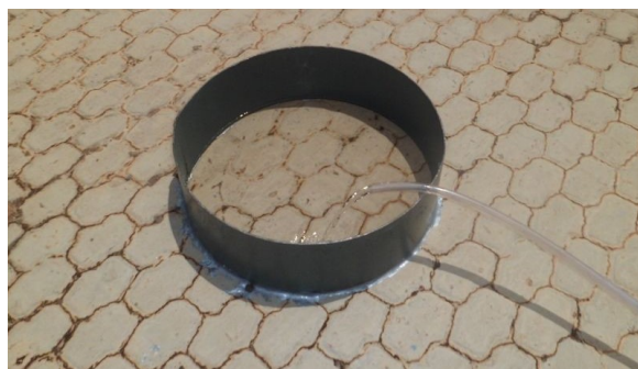
Figure 12. Permeability test on interlocking floors.
