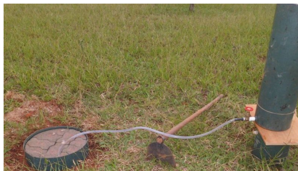
Figure 11. Permeability test on interlocking floors.
