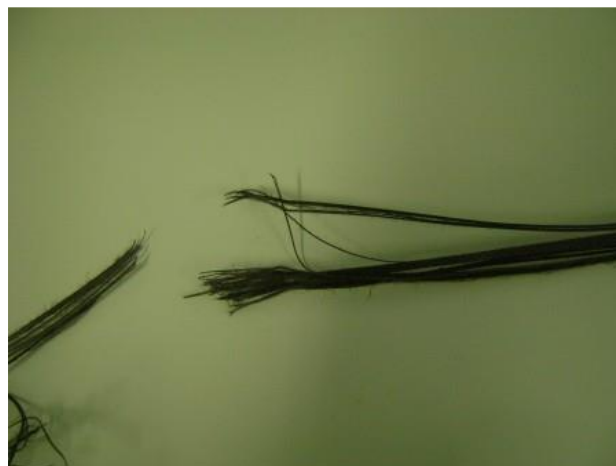
Figure 6. View of the broken tape in the tensile test.
