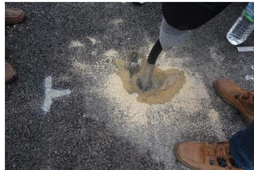
b) cavity wall in sand layer
