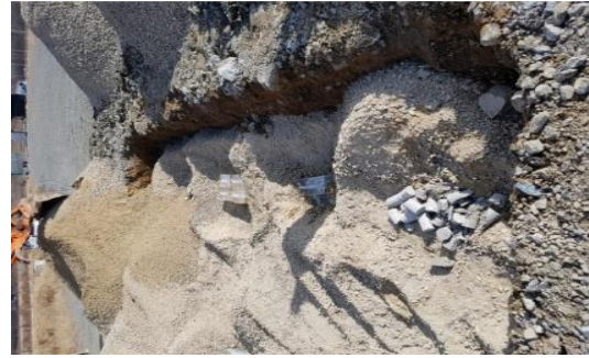
b) Ice for simulating the cavity
