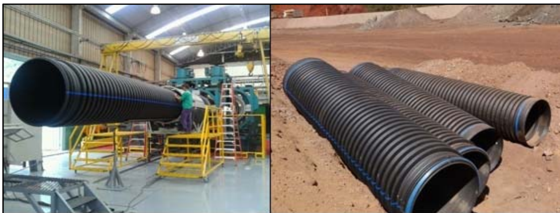
Figure 6. Manufacture and disposal on site of corrugated pipes.
