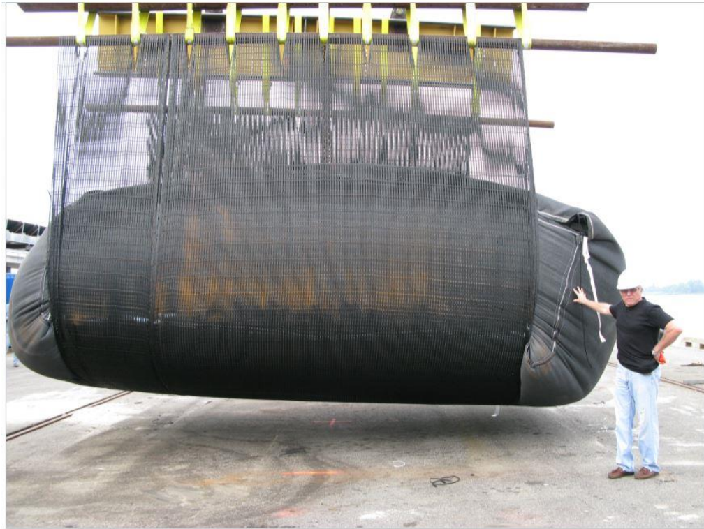
Figure 6 First Test Lifting of the 50 m3 Sand Filled Geobag Container weighing 90 Metric Tons
