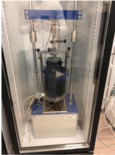
Fig. 8. Test apparatus according to GOST 28622-2012 standard
