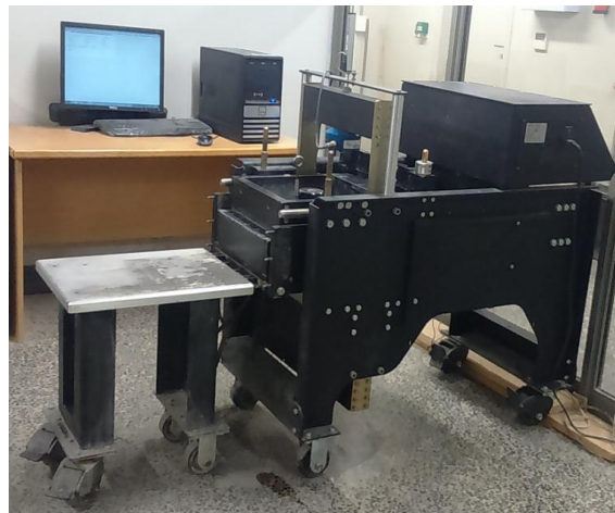
Figure 4. Interface direct shear strength test equipment.
