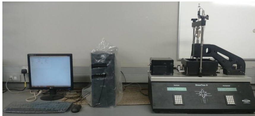
Figure 2. Direct shear test equipment.
