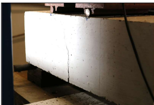
(a) Crack initiation and propagation
