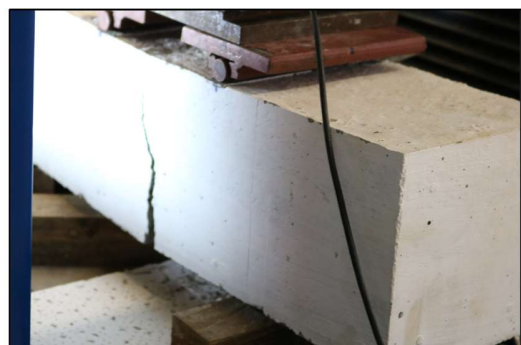
(b) failure mode in reinforced beam
