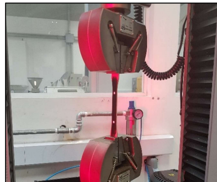
d) Injected test specimens during test
