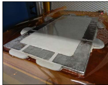
b) Pressed fibers in the form of plate
