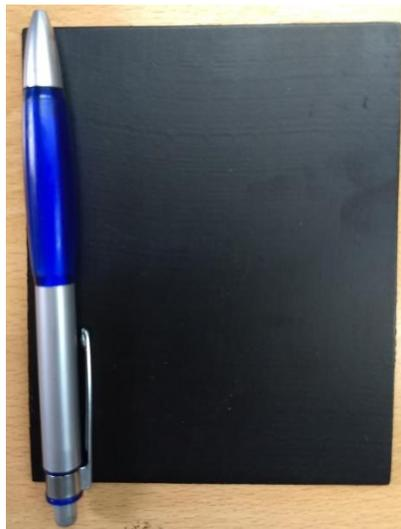
Figure 1: Picture of the tested 1.5 mm thick HDPE smooth geomembrane.
