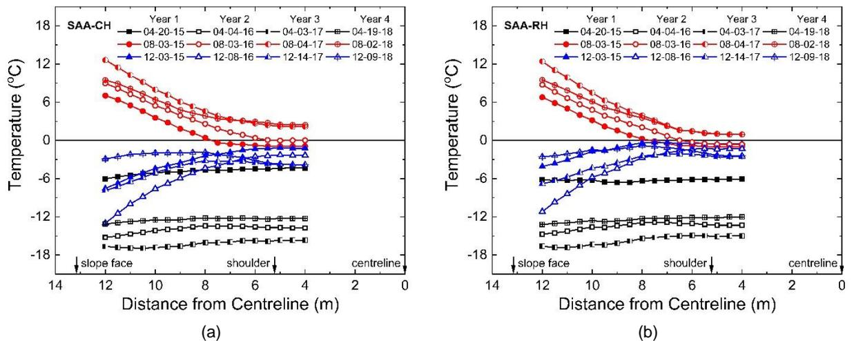
Figure 9. Temperature readings from horizontal SAAs: (a) control section and (b) reinforced section.
