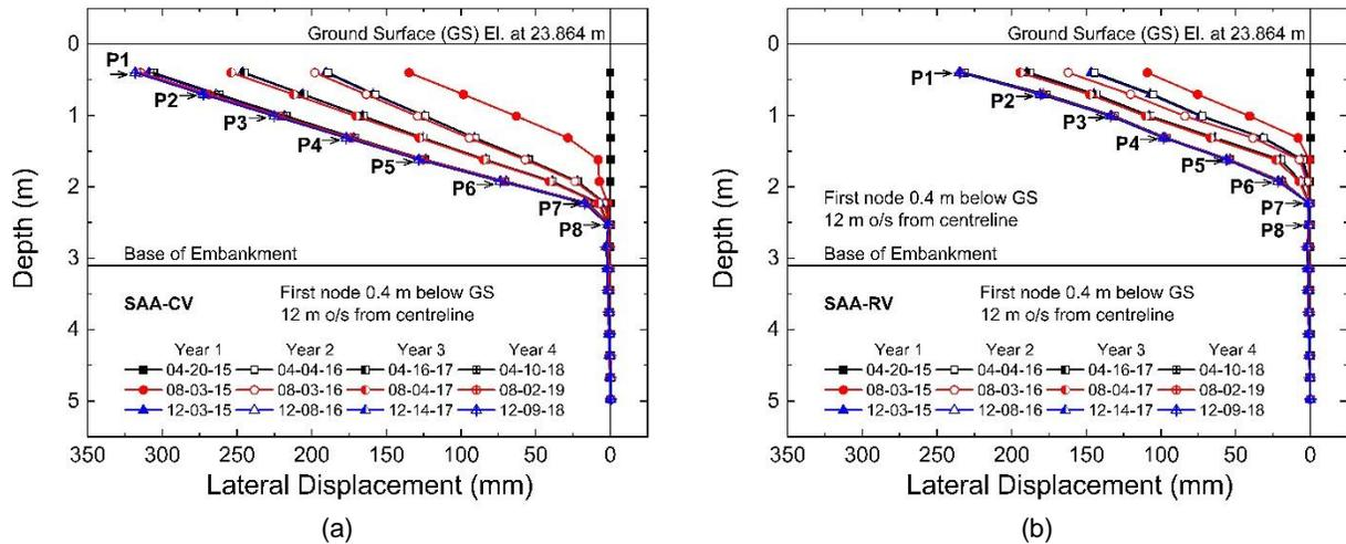
Figure 10. Lateral displacements at midslope: (a) control and (b) reinforced sections.
