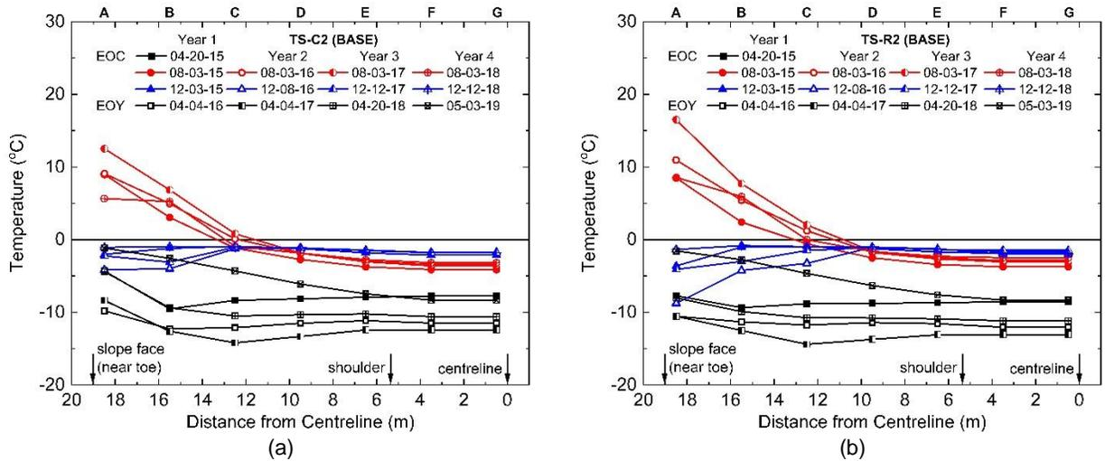
Figure 5. Temperature readings at the base of the embankment: (a) control section and (b) reinforced section.
