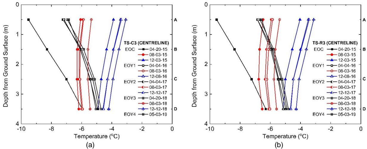
Figure 6. Temperature readings at the foundation centreline: (a) control section and (b) reinforced section.
