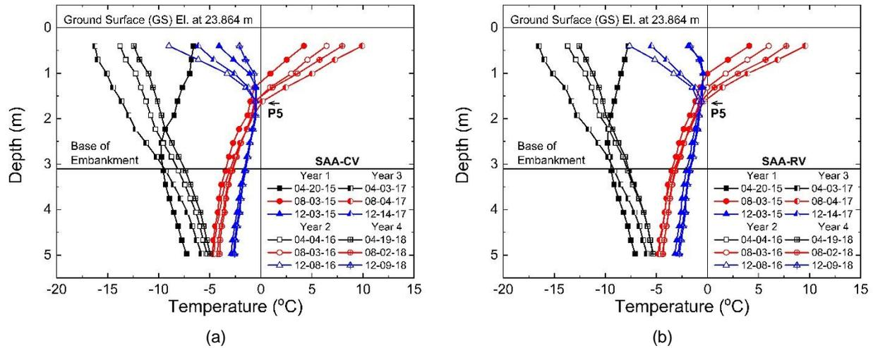
Figure 8. Temperature readings from vertical SAAs: (a) control section and (b) reinforced section.
