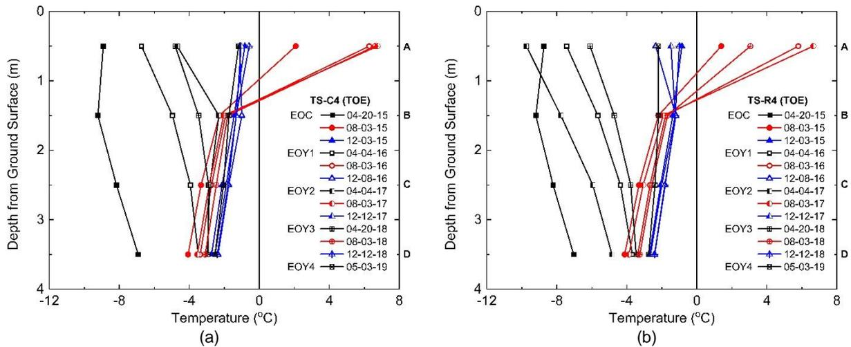
Figure 7. Temperature readings at the toe of the embankment: (a) control section and (b) reinforced section.
