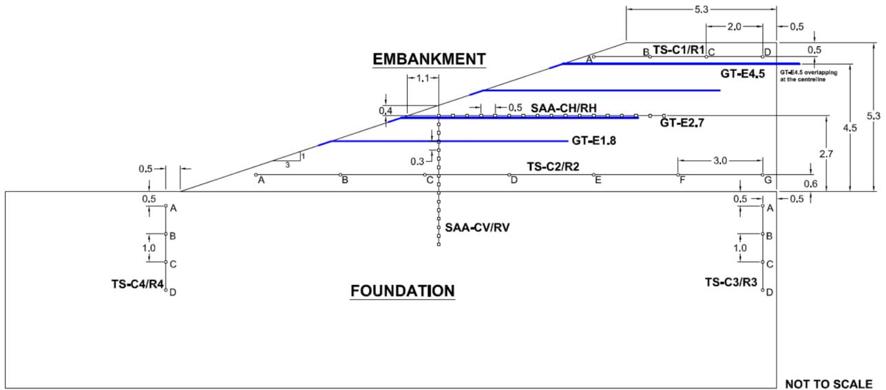
Figure 1. Cross-section of high-fill section with wicking geotextiles, thermistor strings and SAAs. All units in metres.
