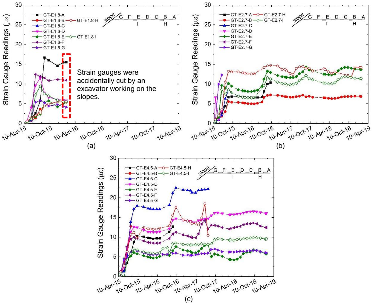
Figure 12. Strain gauge readings with time at different locations: (a) 1.8 m, (b) 2.7 m, and (c) 4.5 m from embankment base.
