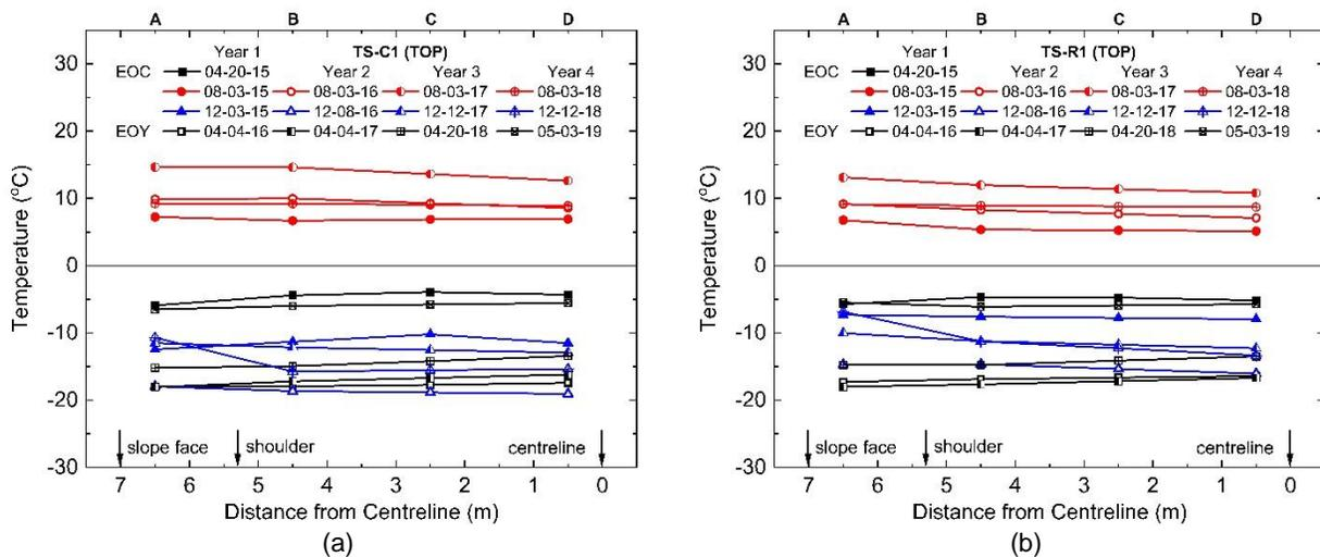
Figure 4. Temperature readings at different time steps at the top of the embankment: (a) control section and (b) reinforced section.
