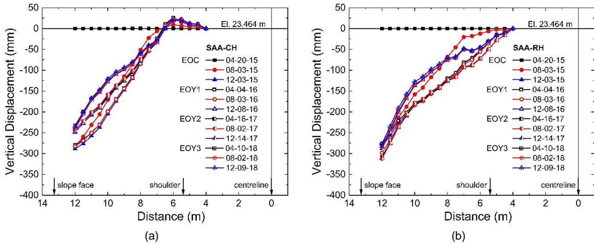
Figure 11. Vertical displacements at midslope: (a) control and (b) reinforced sections. EOC: end-of-construction and EOY: end-of-year.
