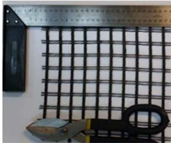
Figure 5. Geogrid used in the study (Góngora 2015)
