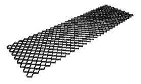
a) 3D view of expanded panel of geocells
