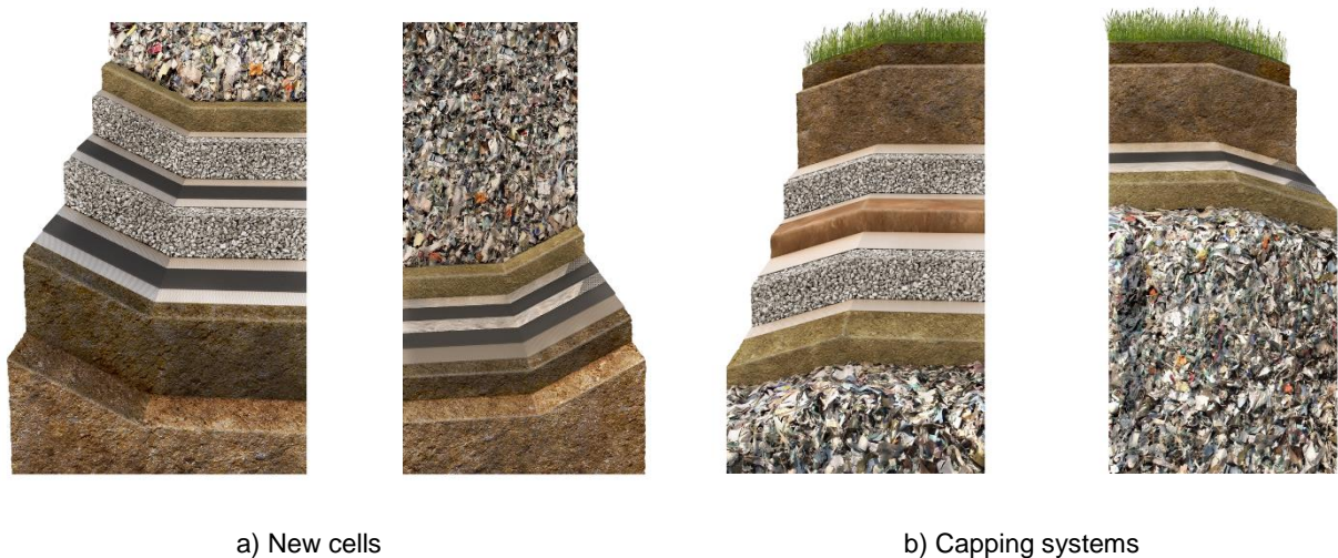
Figure 6. Cross-sectional view comparison between the conventional solution based on a layer of granular material (left) and the geosynthetic design (right). Source: Intermaas Nets.
