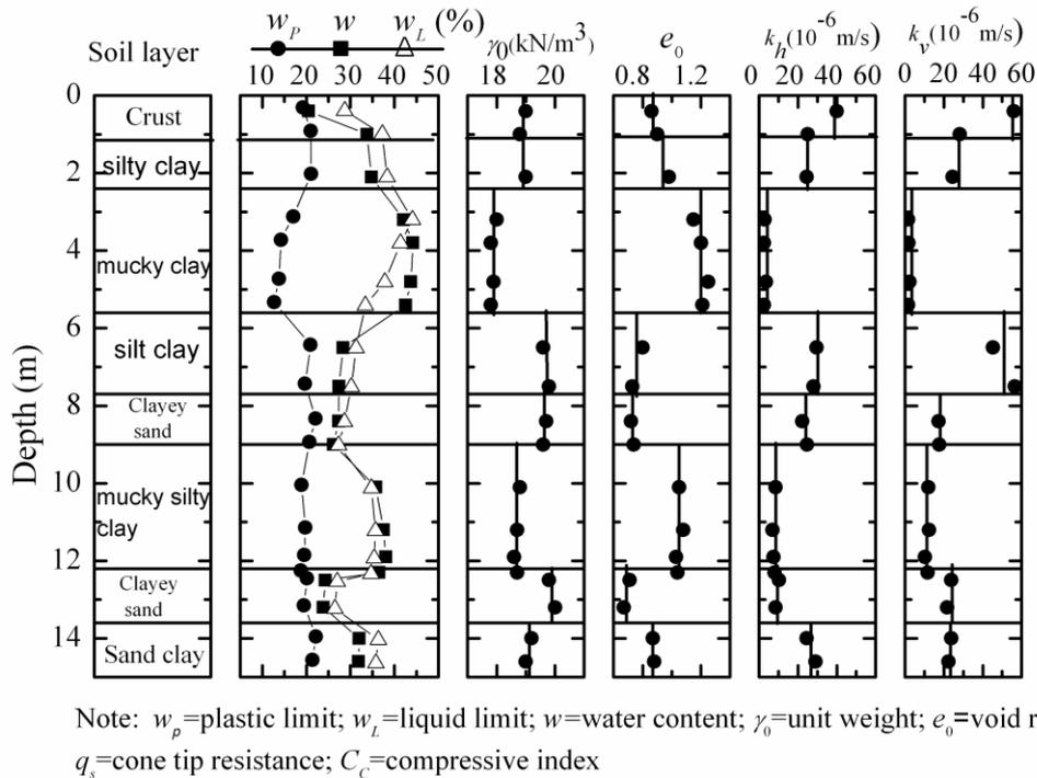
Fig. 1 Soil profile and properties at the test site
