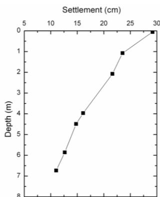
Fig. 6 Settlement vary with depth at the end of embankment construction
