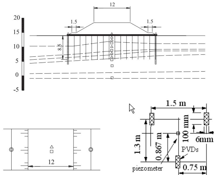
Fig. 2 Cross-section and plan view of embankment, field instrumentation and arrangement of PVDs in field
