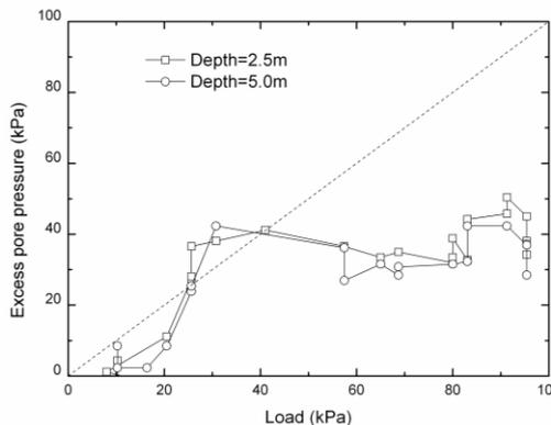
Fig. 9 Pore pressure measured under the centre of the embankment test section as a function of the embankment load
