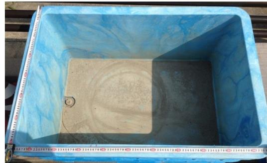
(a) Large-scale model tank with dimension of 1000 mm×650mm
