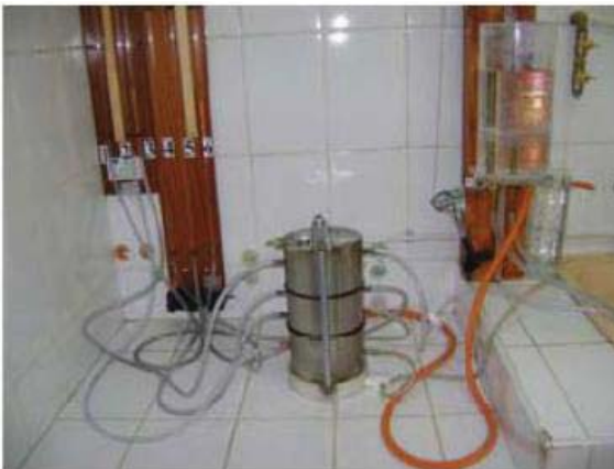
Fig. 3 Apparatus for permeability and clogging capacity testing
