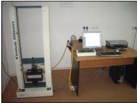
Fig. 1 Apparatus for tensile strength and elongation at break testing
