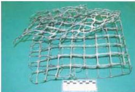
Fig. 6 Geosynthetic sample extracted from the studied railway embankment (Țenea 2007)
